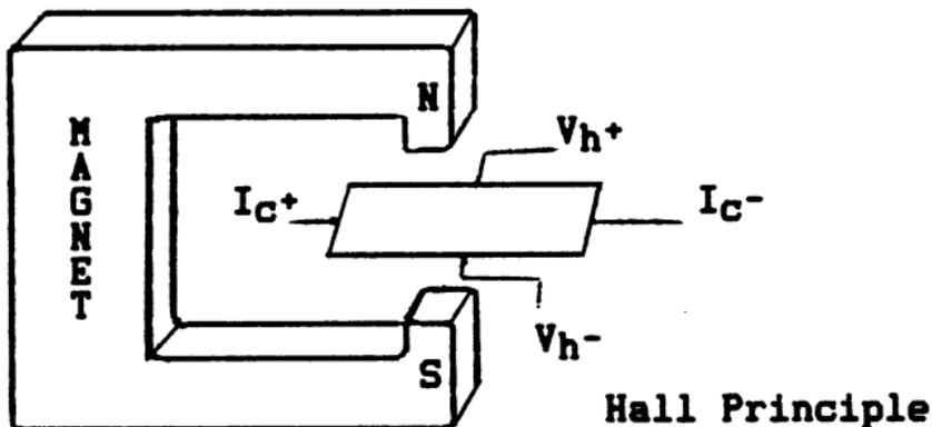
In the Hall layer, electrons deflected to one side result in a charge build-up on that side, and a depletion of charges on the other side. This difference is detected as the Hall voltage, measured at the  $V_h$  terminals.
